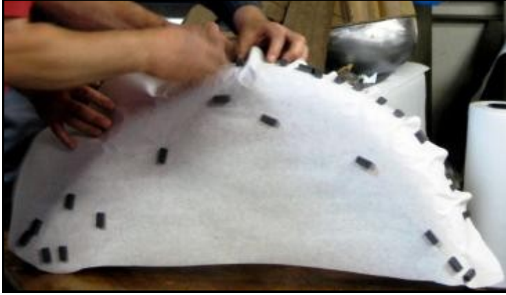
Above left: Tucks following the curvature of a fender. Magnets hold the thin paper sheet to the metal fender allowing the identification of areas of changing shape/curvature. At right: A radius gauge used to determine the radius of curvature of changes in the shape of the fender.
