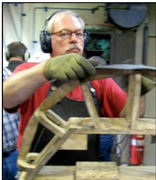
Fay Butler working on form on an Indian fender buck
