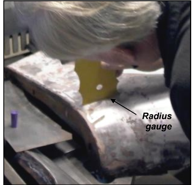
Above left: Tucks following the curvature of a fender. Magnets hold the thin paper sheet to the metal fender allowing the identification of areas of changing shape/curvature. At right: A radius gauge used to determine the radius of curvature of changes in the shape of the fender.
