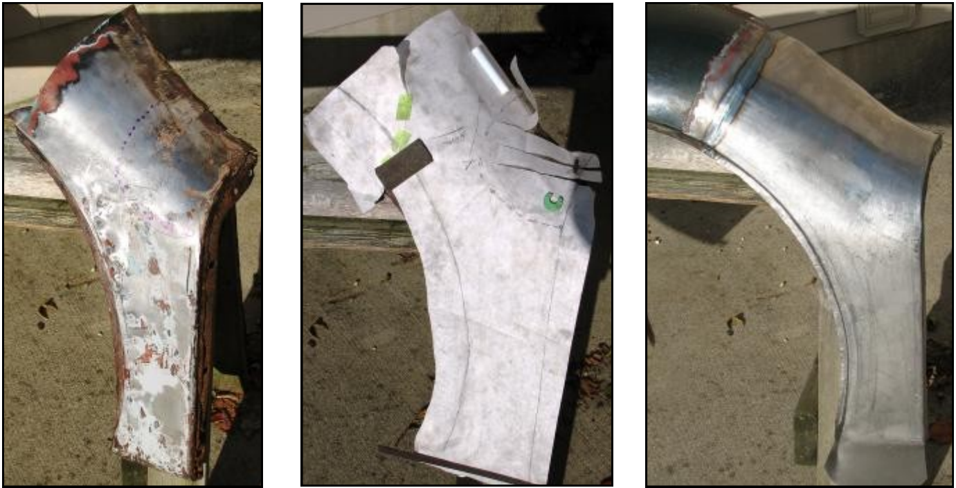
Progression of fender fabrication: from left, the original portion of fender to be remade. Middle: the pattern and fitting on the old fender and at right the finished fender panel attached to the original fender.
