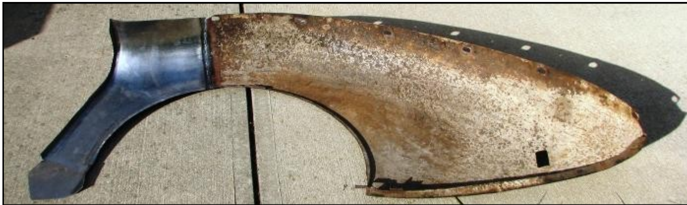
The fender, viewed from the inside, with new attached to old, ready for further restoration.
